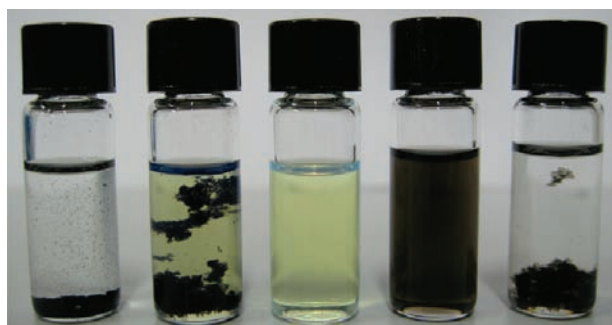
Figure 1. Mixture in \text{CHCl}_3 containing, from left to right, (a) MWCNTs, (b) MWCNTs and 1b , (c) polymer [\mathbf{1b}\cdot\mathbf{2}]_n , (d) hybrid MWCNTs• [\mathbf{1b}\cdot\mathbf{2}]_n and (e) MWCNTs, 1b and 2 after addition of DMSO.
